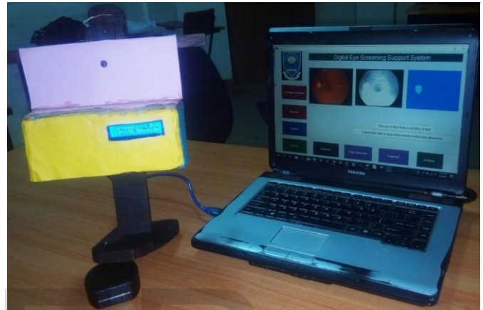
Figure 4: The Final Prototype of the eye screening support system.
